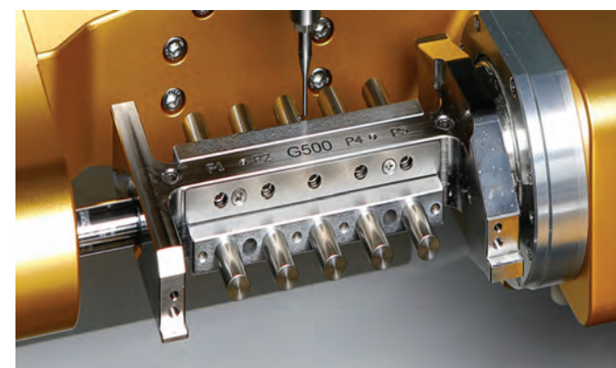
Wireless Auto Calibration improves the usability and accuracy, maintaining the best machining condition.
