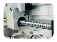
Superior dynamic motion and positional accuracy thanks to large-diameter C5 class precision ball screws. anti-backlash ball nuts and linear guides with closed loop servo drives.
