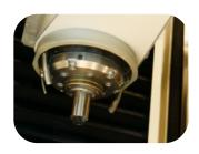
High-torque, 2.7kW max liquid-cooled spindle with 3 ceramic hybrid bearings that help to reduce margin thickness, and extend spindle life by reducing deflection and protecting against contamination by cutting chips and coolant.
