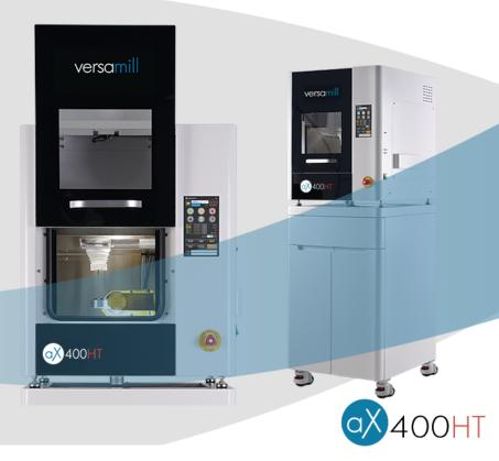
The Versamill AX400HT is a compact 5-axis dental machining center designed for the wet or dry precision machining of copings, crowns, bridges, dentures, titanium custom abutments, models and more.
