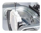
Labial (or Buccal) side texture and undercut area precision processing minimize post-processing time. You can easily exchange from disk to CAD block as it uses cartridge type materials.
