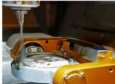
Zirconia sludge (the mixture of zirconia and water) is by far easier to deal with than dry zirconia dust, does not infiltrate machine components and is significantly less destructive to machine components than caustic and abrasive dry zirconia swarf (by-products of the machining process).
