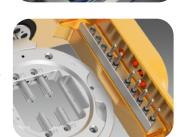
Quick-change 6-unit CAD-block cartridge. Facilitates light-duty production of lithium disilicate, Lava Ultimate and other pre-mounted dental material.
